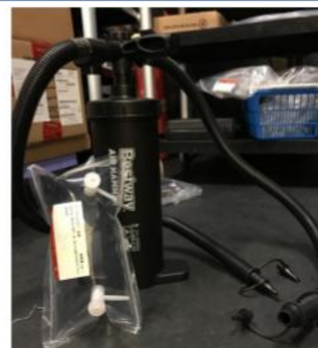
Fig. 2 An picture of the pump and the Tedlar sampling bag
