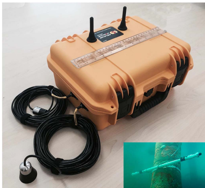
Fig. 2. This photo shows the ShotSpotter sensor rehoused in a plastic case. Hydrophones and cables are shown before being installed in booms. The inset on the lower right shows the hydrophones in their boom and mounted underwater.
